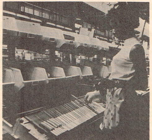
On the control panel assembly line, subassemblies move from station to station. LEWISystems assembly units make parts readily available and can be changed quickly if product assembly is altered.
