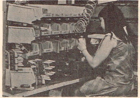
Handy finger-tip convenience of parts speeds up assembly functions of control tab subassembly. Circular arrangement of bins allows easy access.
